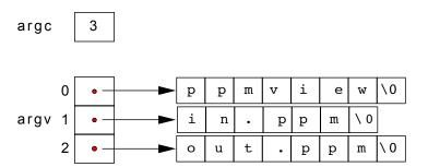
Figure 2.6: argc and argv data structures in C
